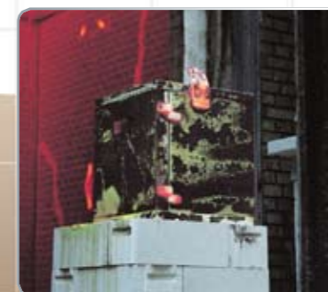
Removal of cabinet from oven
